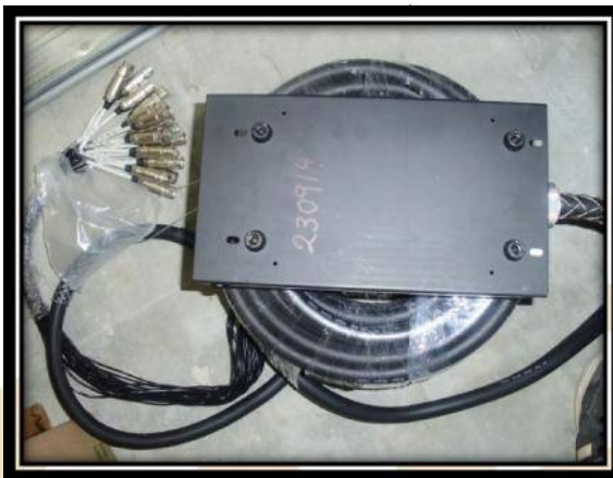
Consola SNAKE-RSW16C35-SNAKE 16CH.4 RET SWITCHCRAFT 35M SOLCOR
